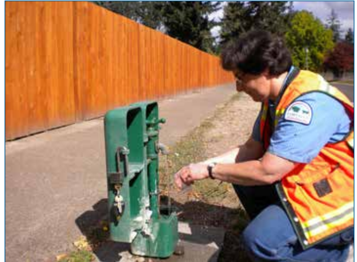
Water Quality Analyst Cris Piccioni collects a sample from the distribution system.
